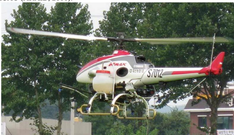
**Figura 1.5** – Unmanned Rotorcraft Yamaha RMAX L17 (ARAIB, 2010).
